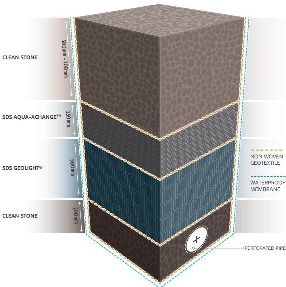
SDS Aqua-Xchange™ is a granular material suitable for use in devices where stormwater can percolate through the material, allowing sufficient contact time for the pollutants to be captured.
