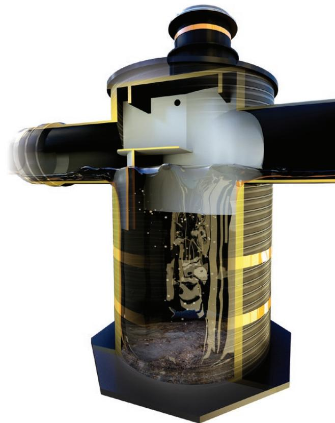
SDS Aqua-Swirl™ is sized according to water quality treatment flow rates which are based on the initial movement of pollutants into the storm drainage system. This flow rate typically represents approximately 90% to 95% of the total pollutants in the runoff volume.
