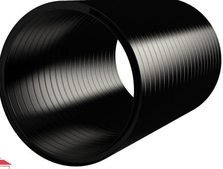
The uniqueness of the Weholite production process means that pipes can be run in any length from 300mm to 30m in one piece. It is one of the few polyethylene pipes in the world that can be produced in dimensions larger than two metres and can be supplied in ring stiffness classes from 2 to 8kN/m².
